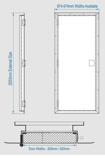
Our Standard Duty Steel Personal Access Doors are made of 0.8mm galvanised steel door skins and 1.4mm galvanised frames, and they come with three stainless steel ball-bearing hinges. Polyurethane foam (also known as PU foam) is injected into the door leaf for increased insulation and rigidity, and 3 stainless steel butt hinges hold the leaf in the frame.
