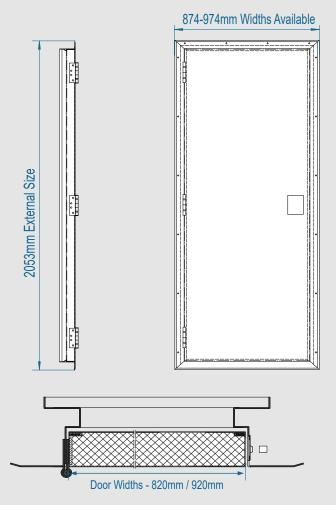
Our Standard Duty Container Doors are made of 0.8mm galvanised steel door skins and 1.4mm galvanised frames, and they come with three stainless steel ball-bearing hinges. Polyurethane foam (also known as PU foam) is injected into the door leaf for increased insulation and rigidity, and 3 stainless steel butt hinges hold the leaf in the frame.
