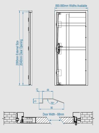
Featuring thicker gauge steel, a denser core and an extra hinge compared to our single steel door, this is a great option for an affordable steel security door.
