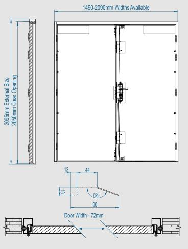
These doors are manufactured from galvanised steel with a fully welded construction, as well as a heavy duty polyester powder coat. They are also fitted with weather and draught-proof seals making our steel doors ideal for both internal and external uses such as garages, shops, commercial premises and modular buildings.
