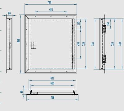
Our container access hatches are perfect for container conversions and modifications. Made from galvanised steel, they have a fully welded frame with sealed joints and very simple to face fix into a shipping container.
