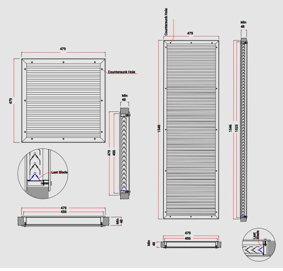
Steel welded box section frames are required to weld the louvre within.
