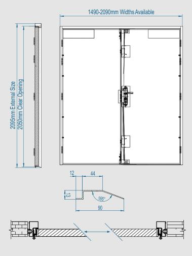
Our Double Steel Air Vent Doors are pre-installed with air relief grilles to promote airflow and ventilation whilst maintaining a high level of security. Offering up to 50% air flow, they are suitable for boiler rooms, plant rooms and server rooms.
