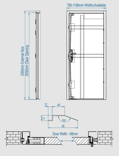
Made from galvanised steel and including our HOOPLY™ 19-point locking system as standard.
