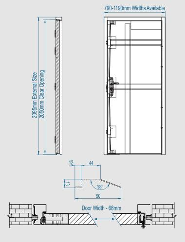
This door has been designed with security in mind, and is ideal for securing any type of property, as compared to our standard duty version.
